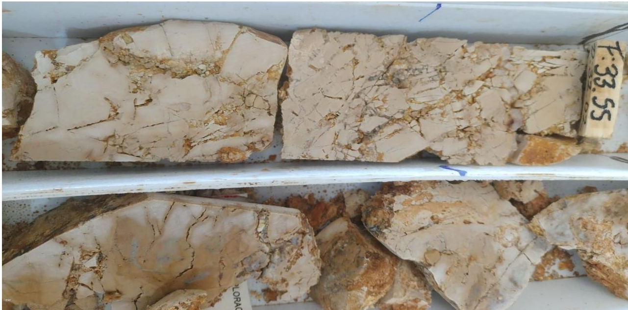
Figure 4. 30cm core at TDD-001 33m: Ex-sediment, crackle breccia, completely clay altered, moderately silicified with broken stockwork quartz veinlets.
