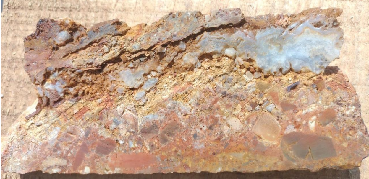
Figure 1. 20cm core at TDD-001 19m: Oxidized silicified polymict hydrothermal breccia with stockwork banded veining.
