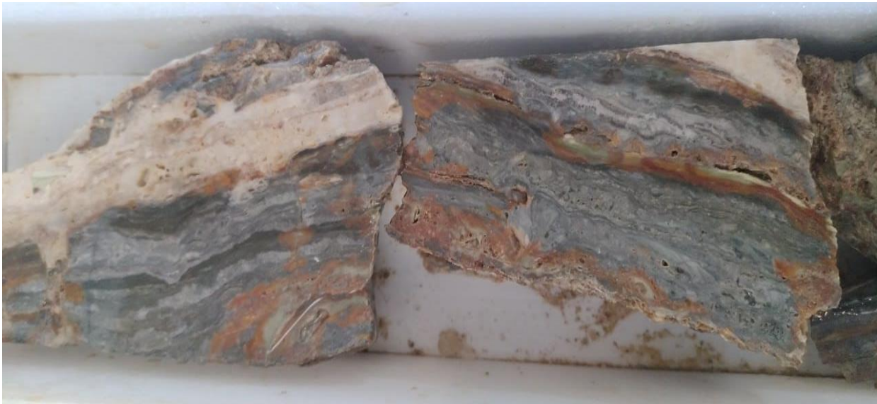
Figure 5. 20cm core at TDD-001 53m: Banded quartz veining with strong fine grained dark sulphides.
