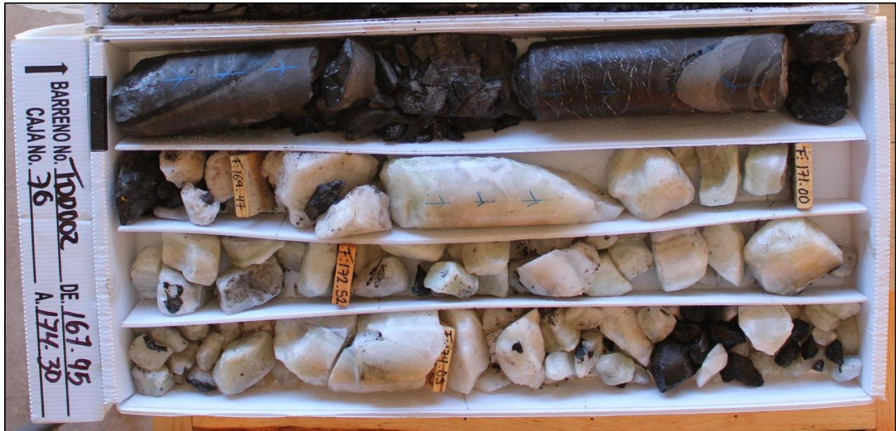
Figure 7. TDD-002 at 168m to 174m: Banded chalcedonic quartz vein.
