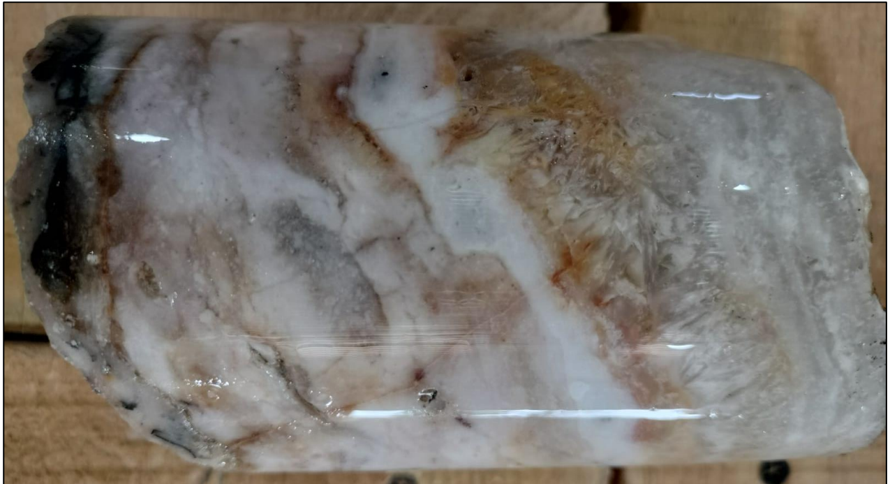
Figure 3. TDD-003 at 66m: 10cm of banded chaledonic quartz vein
