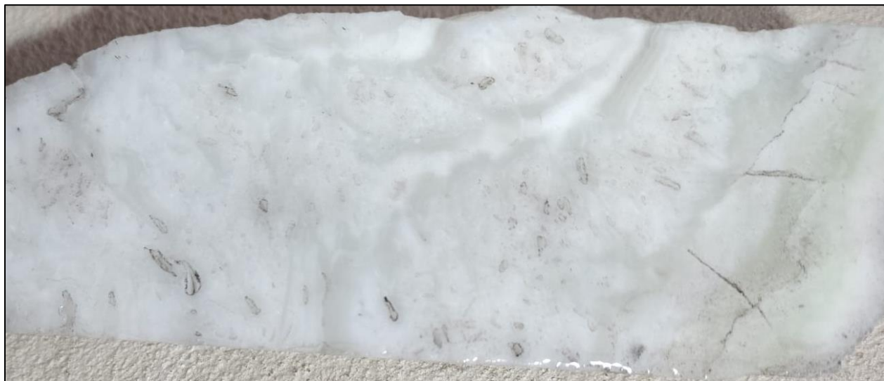
Figure 6. TDD-002 at 169m: 10cm Banded chalcedonic quartz vein
