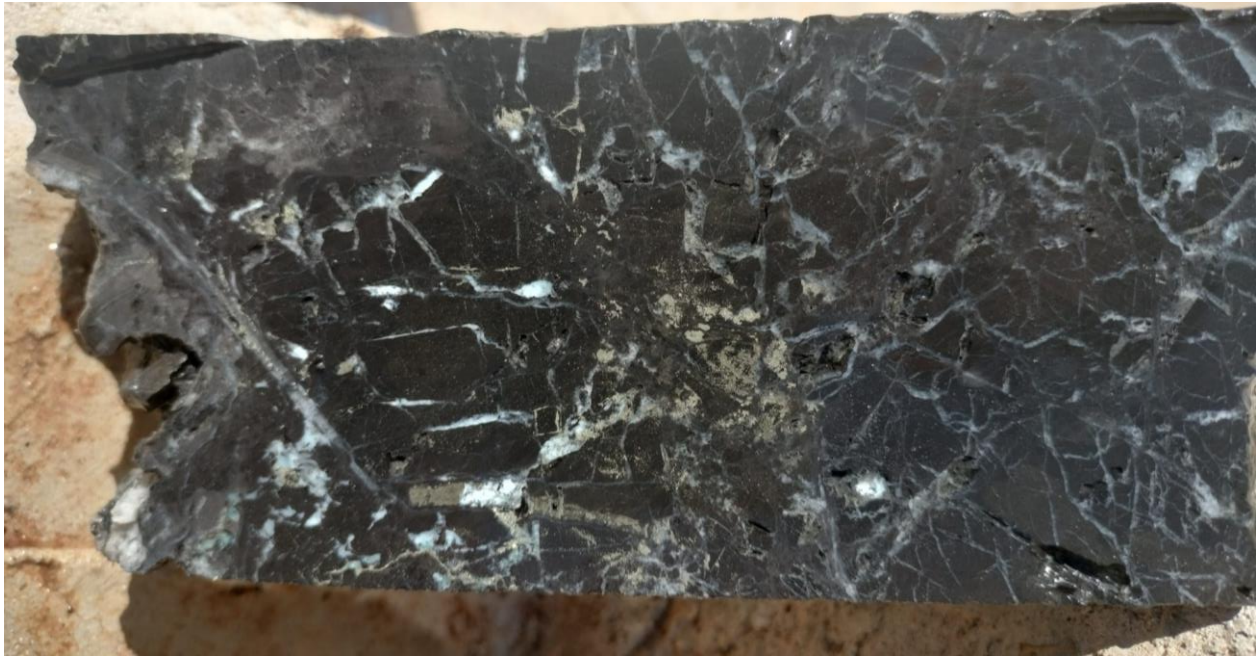
Figure 5. TDD-002 at 83m: Silicified cataclasite (faulted and crushed pelite sediment) with abundant pyrite.
