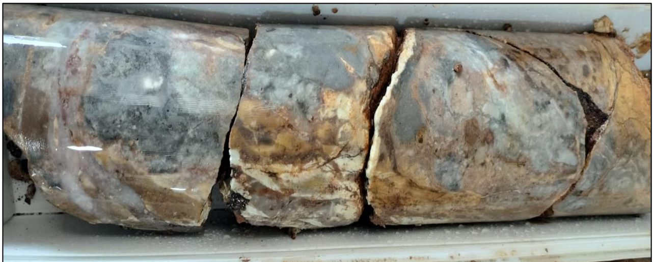
Figure 2. TDD-003 at 27m: 30cm of intensely silicified breccia
