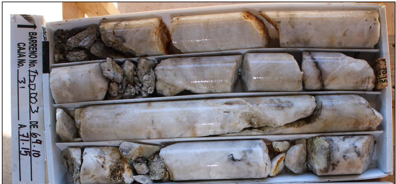
Figure 4. TDD-003 at 69 to 71m: Banded chaledonic quartz vein and breccia
